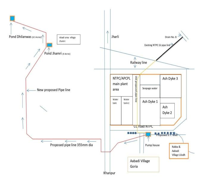
Constructing Goria Pipe Line Link Drain ( Underground Pressurized HDPE Pipe Line) from RD 0 to 10 km
